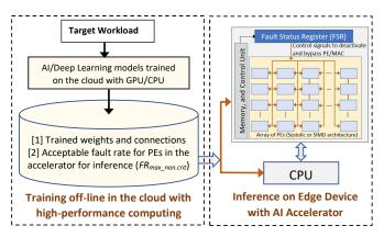
Figure 6: Deactivating some non-critically faulty PEs to keep fault rate within  $FR_{max\_non-crit}$  to ensure accuracy does not degrade beyond acceptable limit.
