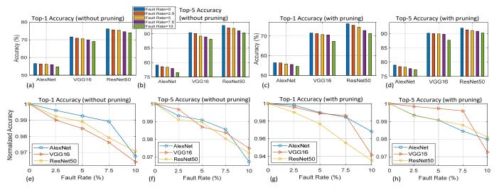
Figure 8: Inference accuracy changes with fault (non-critical) rates for CNNs running imagenet dataset. (a), (b) Top-1 and Top-5 accuracy changes ; (c), (d) Top-1 and Top-5 accuracy changes with model pruning; (e) to (h) normalized accuracy changes in Top-1 and Top-5 (with and without pruning) for fault rates.
