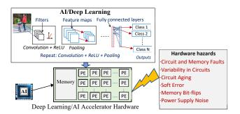
Figure 4: Hardware hazards and faults impacting AI accelerator chips.
