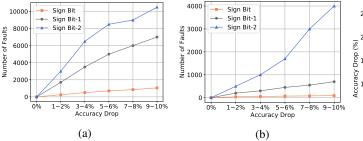
Figure 2: Impact of Faulty Bit Position on Classification Accuracy of MLP on (a) MNIST and (b) Fashion-MNIST.
