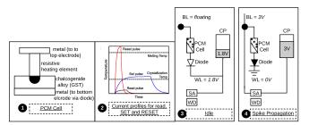
Figure 11: Operation of PCM in neuromorphic computing.
