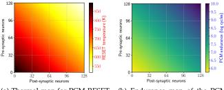
(a) Thermal map for PCM RESET operations in a 128x128 crossbar.
