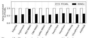
Figure 12: Circuit aging in the neuromorphic hardware normalized to PyCARL (lower is better) [51].
