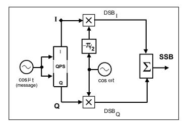
Figure 2: practical realization of the SSB phasing generator
