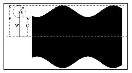
Figure 3 : measuring sideband suppression via the envelope
