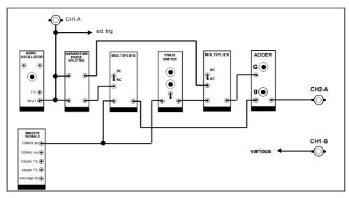
Figure 5: the SSB phasing generator model
