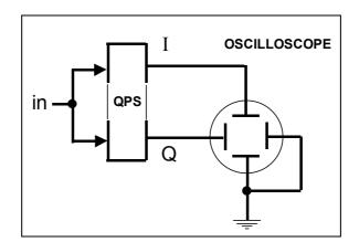
Figure 4: arrangement to check QPS performance
