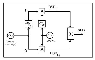
Figure 1: principle of the SSB Phasing Generator
