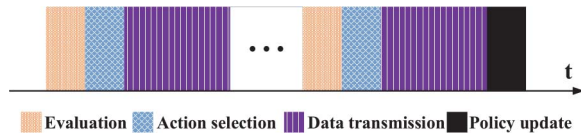
Fig. 2. Time slot model. At the front of each time slot, the current state is first evaluated, the action to be taken (the UAV number to perform information sharing) is then selected, the information is transmitted, and finally the policy is updated at the end of the round.
