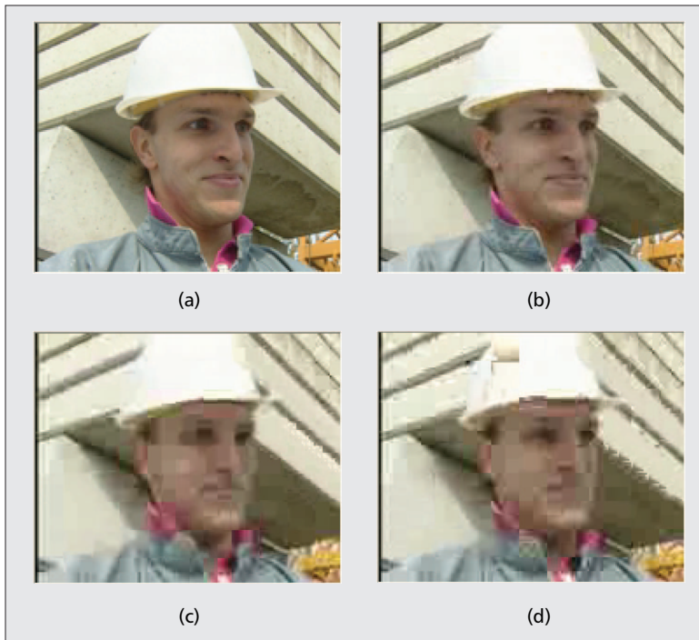
■ Figure 2. Frame 224 from the original and decoded video sequences "Foreman" delivered by different routing algorithms: a) original; b) cross-layer routing; c) 2-SP; d) DPSP.
