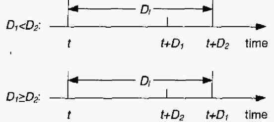
Fig. 4. Determining the end-to-end delay  $D_l$ .
