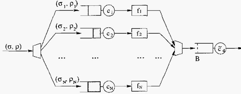
Fig. 7. A traffic partitioning model with  $N$  paths.
