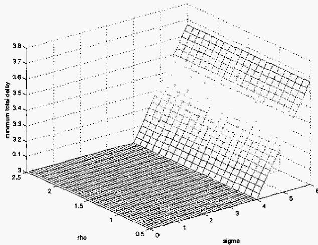
Fig. 13. The minimum end-to-end delays for a two-path system having  $\mathbf{f} = \{1, 3\}$  and  $\mathbf{c} = \{2, 1\}$ :  $\tilde{D}_1^*$ , using (14).
