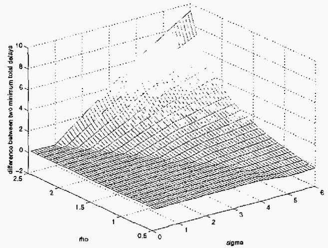
Fig. 14. The minimum end-to-end delays for a two-path system having  $\mathbf{f} = \{1, 3\}$  and  $\mathbf{c} = \{2, 1\}$ :  $D_1^* - \tilde{D}_1^*$ .
