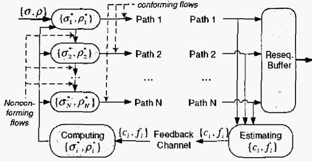
Fig. 11. Implementation of the optimal traffic partitioning scheme.
