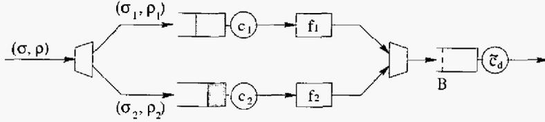
Fig. 2. A traffic partitioning model with two paths.
