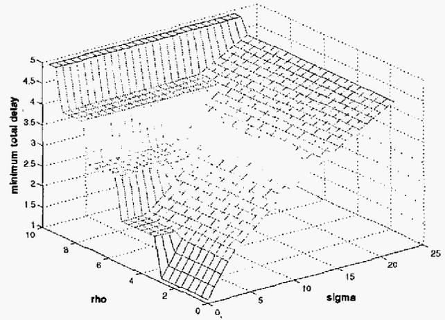
Fig. 15. End-to-end delay and optimal leaky bucket parameters for a five-path system having  $\mathbf{f} = \{1, 2, 3, 4, 5\}$  and  $\mathbf{c} = \{1, 1.5, 2, 2.5, 3\}$ : Minimum end-to-end delay  $D_1^*$ .
