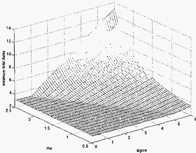
Fig. 12. The minimum end-to-end delays for a two-path system having  $\mathbf{f} = \{1, 3\}$  and  $\mathbf{c} = \{2, 1\}$ :  $D_1^*$ , using (5).
