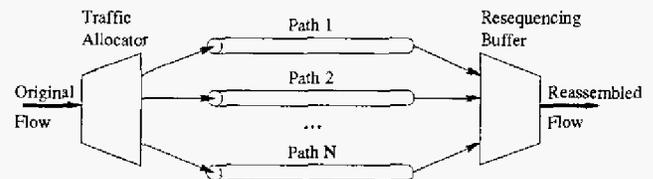
Fig. 1. The general architecture of multipath transport.
