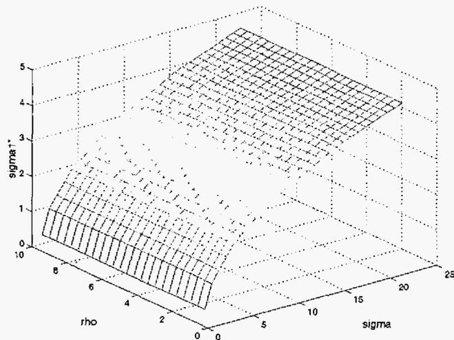
Fig. 16. End-to-end delay and optimal leaky bucket parameters for a five-path system having  $f = \{1, 2, 3, 4, 5\}$  and  $c = \{1, 1.5, 2, 2.5, 3\}$ : Optimal Path 1 burst assignment  $\sigma_1^*$ .
