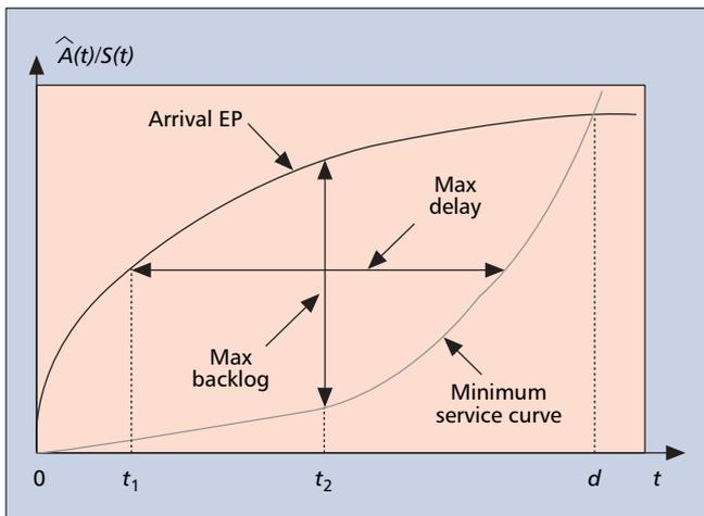
■ **Figure 10.** A graphical interpretation of maximum delay and backlog using the arrival EP and minimum service curve.
