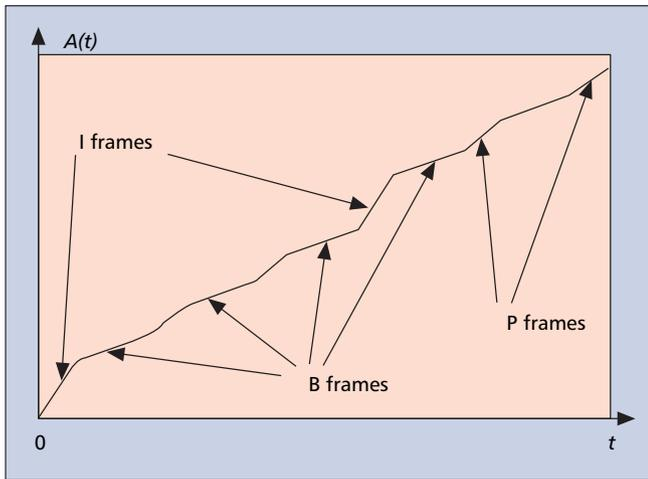
■ **Figure 3.** Burstiness of an MPEG video trace with a frame pattern of IBBPBBPBB.
