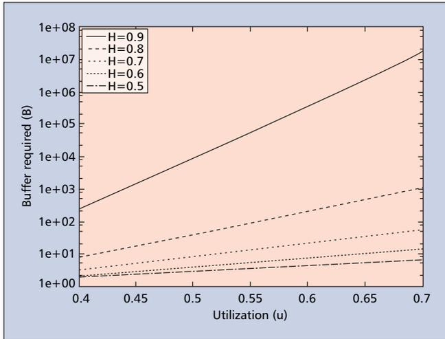
■ **Figure 8.** The trade-off between buffer size ( $B$ ) and utilization ( $u = \rho/x$ ) when using a leaky bucket regulator for fBm traffic.
