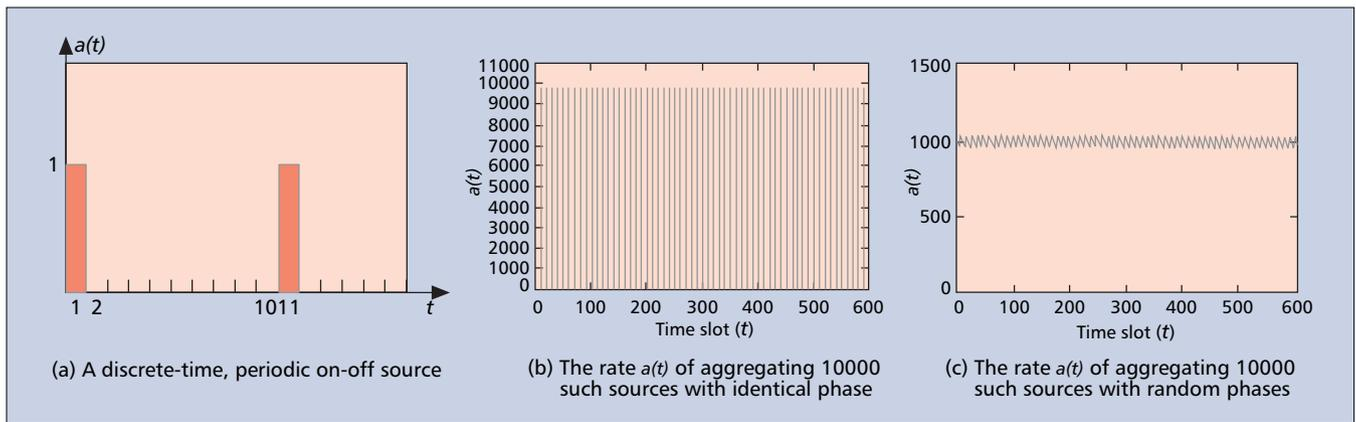
■ **Figure 6.** An illustration of statistical multiplexing gain.
