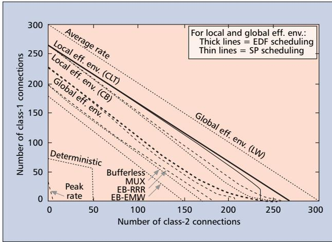
■ **Figure 7.** Admissible region of multiplexing Class 1 and Class 2 flows with  $\epsilon = 10^{-6}$ , delay deadlines  $d_1 = 100$  ms, and  $d_2 = 10$  ms [23]. © 2000 IEEE.
