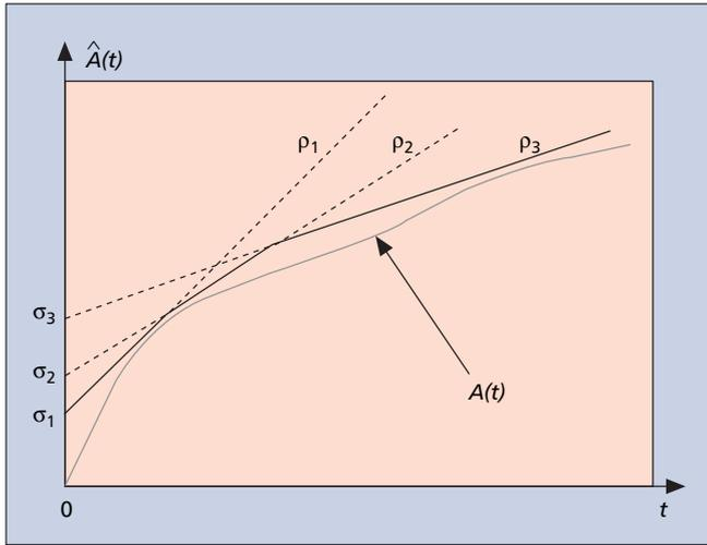
■ **Figure 2.** A piece-wise linear  $\{\hat{\sigma}, \hat{\rho}\}$  envelope process with three  $\{\sigma, \rho\}$  pairs.
