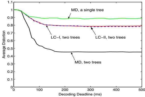
**Figure 5. Effect of the decoding deadline: comparison of four video multicast schemes.**
