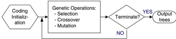
**Figure 4. The GA-based multicast routing.**
