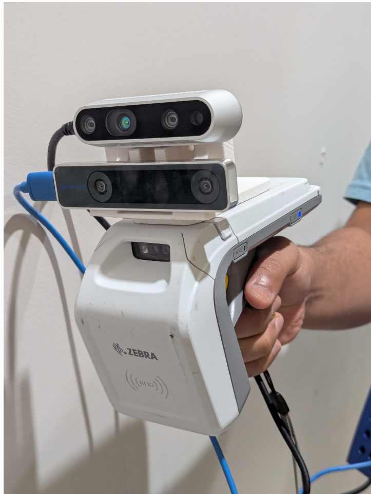
Figure 3.2: The RF-visual sensing component: Realsense D435 RGB-D camera (Top), Realsense T265 tracking camera (Middle), and the Zebra RFD8500 Bluetooth Handheld UHF RFID Reader (Bottom).
