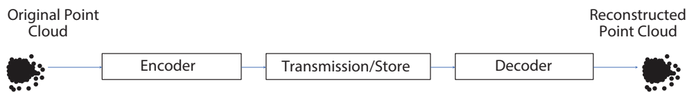
FIGURE 1. The general PCC system structure.
