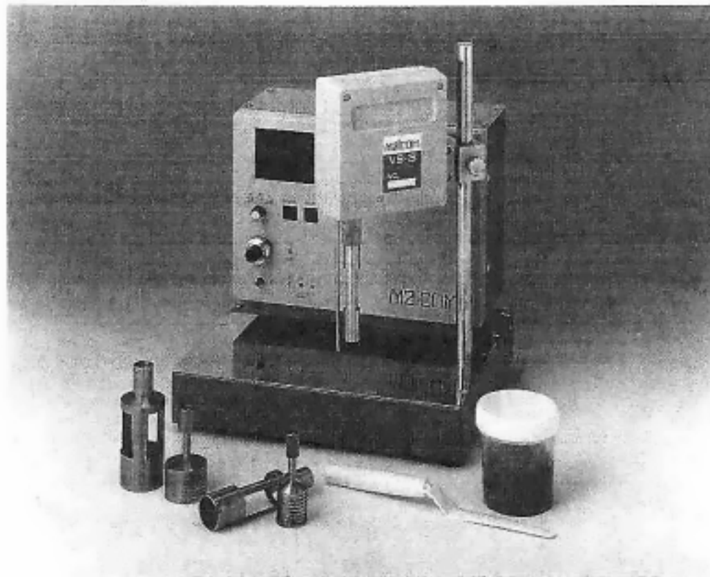
Figure 9.6 Photograph of spiral (Malcom) viscometer. (Courtesy Malcoln Instruments Corporation.)
