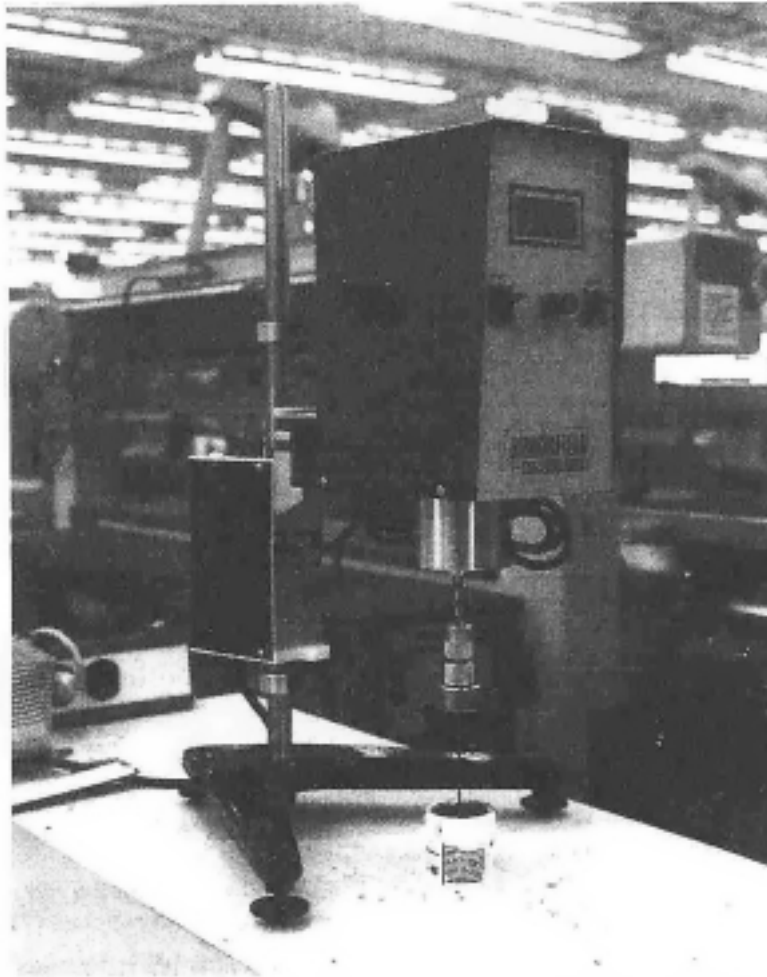
Figure 9.5 Brookfield viscometer. (Photograph courtesy of Intel Corporation.)
