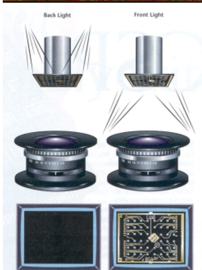
Figure 3. Effect of placement equipment vision system on inspection of bump-array packages. Larger pitch BGAs are typically placed via front lighting with bump-array inspection. Back lighting uses the part outline only to neutralize part-to-part variations.
