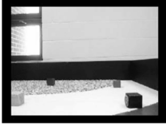
Figure 6. The output from the digital camera. Included in the image are the four blocks to be detected. There is a black background on the rink, there is a blue and white surface, and there are some pebbles.
