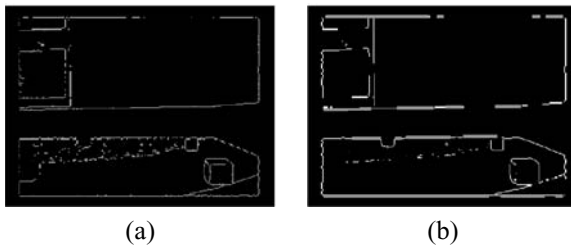
Figure 7. (a) Magnitude of the x and y gradients using the Sobel kernels. (b) Lines extracted from the Hough transform plotted on top of the Sobel edge detection in (a).
