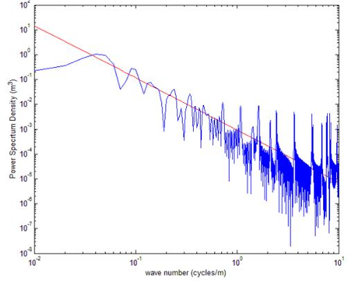
FIGURE 2. PSD OF GENERATED FRACTAL SURFACE COMPARED TO IDEAL PSD FRACTAL LINE.
