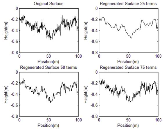
FIGURE 4. SURFACES DECOMPOSED USING FFT AND REGENERATED WITH DIFFERENT NUMBERS OF FOURIER COEFFICIENTS
