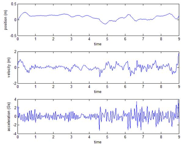
FIGURE 11. VEHICLE RESPONSE OF SPRUNG ( $z_s$ ) MASS WHEN DRIVING OVER SURFACE WITH A CHANGE IN ROUGHNESS
