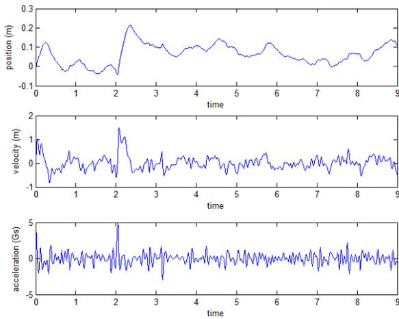
FIGURE 9. VEHICLE RESPONSE OF SPRUNG MASS ( $z_s$ ) WHEN DRIVING OVER PROFILE WITH A STEP INCREASE
