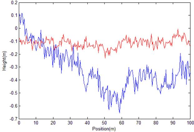
FIGURE 1. RANDOMLY GENERATED 2D TERRAIN PROFILES FOR MILD PROFILE (RED) AND ROUGH PROFILE (BLUE)
