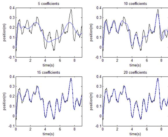
FIGURE 6. POSITION OF SPRUNG MASS FOR SIMULATIONS OVER REGENERATED SURFACES WITH DIFFERENT NUMBERS OF FOURIER COEFFICIENTS.
