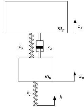
FIGURE 3. 2 DOF QUARTER CAR MODEL USED FOR VALIDATION OF TERRAIN CHARACTERIZATION.
