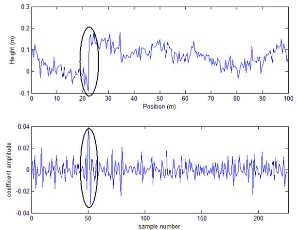
FIGURE 8. PROFILE WITH A DISCONTINUITY WHICH HAS BEEN DECOMPOSED INTO ITS HIGH FREQUENCY COMPONENT USING THE WAVELET TRANSFORM
