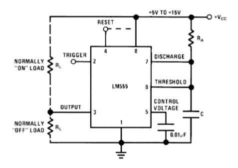
The output is initially low and the trigger input is initially high. Application of a negative going trigger pulse, less than  $V_{cc}/3$ , starts the process. At this time, the output goes high. When  $t=1.1R_AC$ , the output goes back low and stays low until another trigger pulse is applied. The time of the pulse is due to the voltage across C growing exponentially through  $R_A$ .
