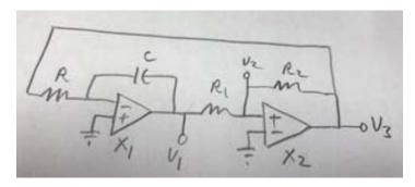
V<sub>3</sub> is a square wave output signal. The oscillation frequency is:
