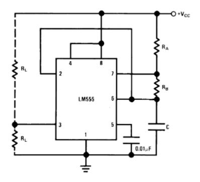
Capacitor C continually charges and discharges between 1/3 V<sub>CC</sub> and 2/3 V<sub>CC</sub>. The output is high during the charge time, which is determined by  $t_c = 0.693$  ( $R_A + R_B$ )C.
