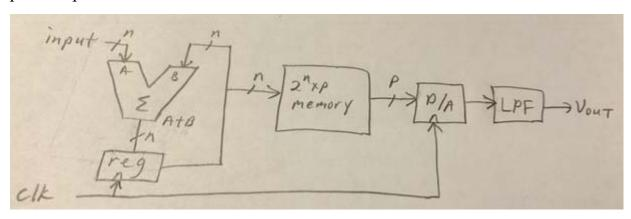
If input is 1, it takes  $2^n$  clk cycles to go through (read out) the entire memory. The frequency of the output sinewave will then be  $f_{CLK}/2^n$ . As the input number increases, it takes fewer clk cycles to go through the address space of the memory, proportionally increasing the frequency of the output sinewave. The LPF is needed to reduce high frequency noise and to smooth the output sinewave. The output sinewave is directly digitally synthesized, hence the name "DDS."
