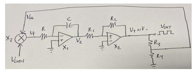
$V_{cntrl}$  is a small DC control voltage and  $V_{cntrl} > 0$  V.
