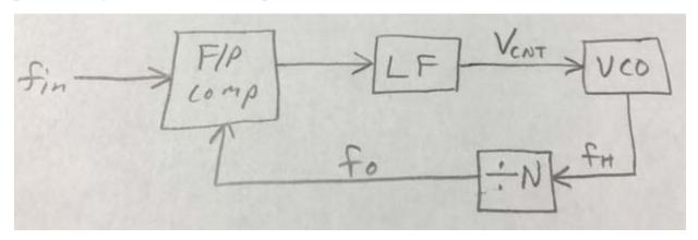
F/P comp: frequency / phase comparator – produces a signal indicating the frequency and/or phase difference between the two input periodic signals. Implementations include four quadrant multipliers, mixers, and logic circuits
