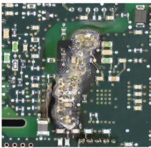
Electrical Shorting Failures
