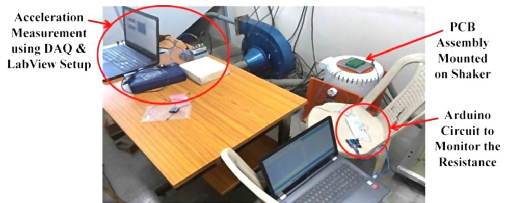
Fig. 6 Random vibration setup
