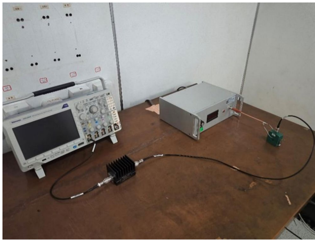
Fig. 5 Experimental platform of HEMP pulse source calibration test circuit
