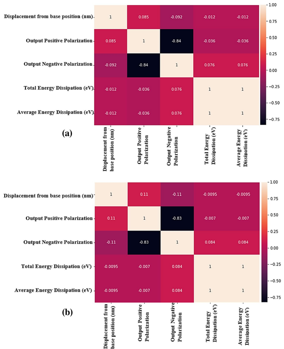
Fig. 11 Correlation matrices to represent the dependencies of predictors and responses in case of a LT NAND and b LT NOR gates
