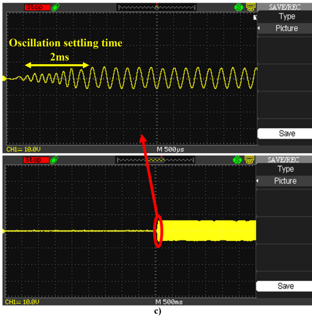
Fig. 5 Oscillation start and settling times of wien bridge oscillator circuit realized with different op-amp models; a traditional op-amp model (simulation result), b proposed op-amp model (simulation result), c tra-
