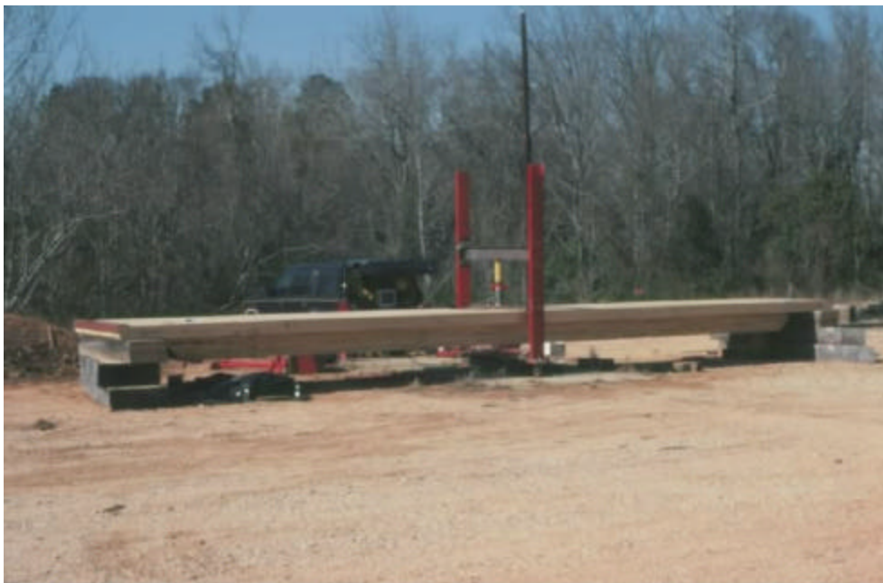
Figure 10. Static bending test of bridge modules at the laminating plant.
