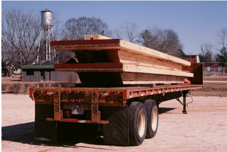
Figure 3. Finished T-section glulam deck modules in preparation for shipment to preservative treatment plant.
