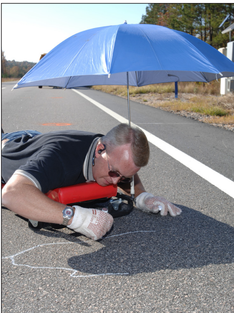
(Left) Test Track Manager Buzz Powell maps cracks on the NCAT Pavement Test Track.
