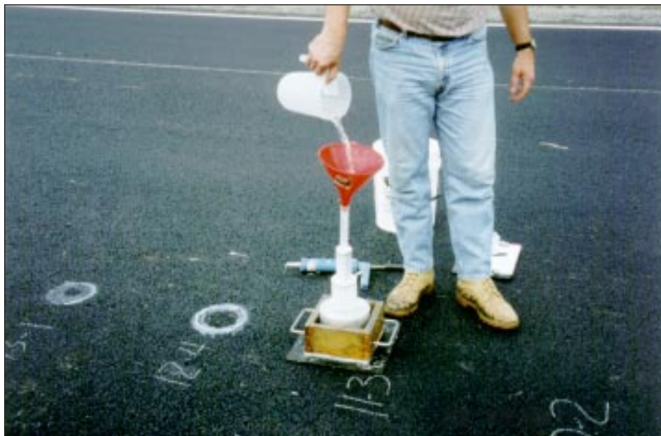
Photo 1. NCAT field permeability device is in use on a new Superpave mix pavement.
