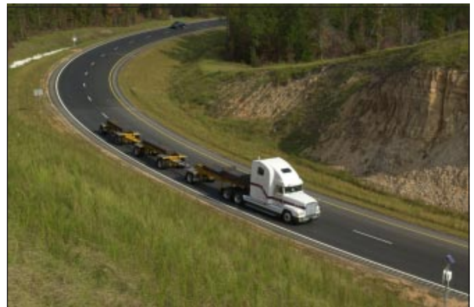
Loading of the NCAT Test Track with four tractor/trailers like the one shown here.
