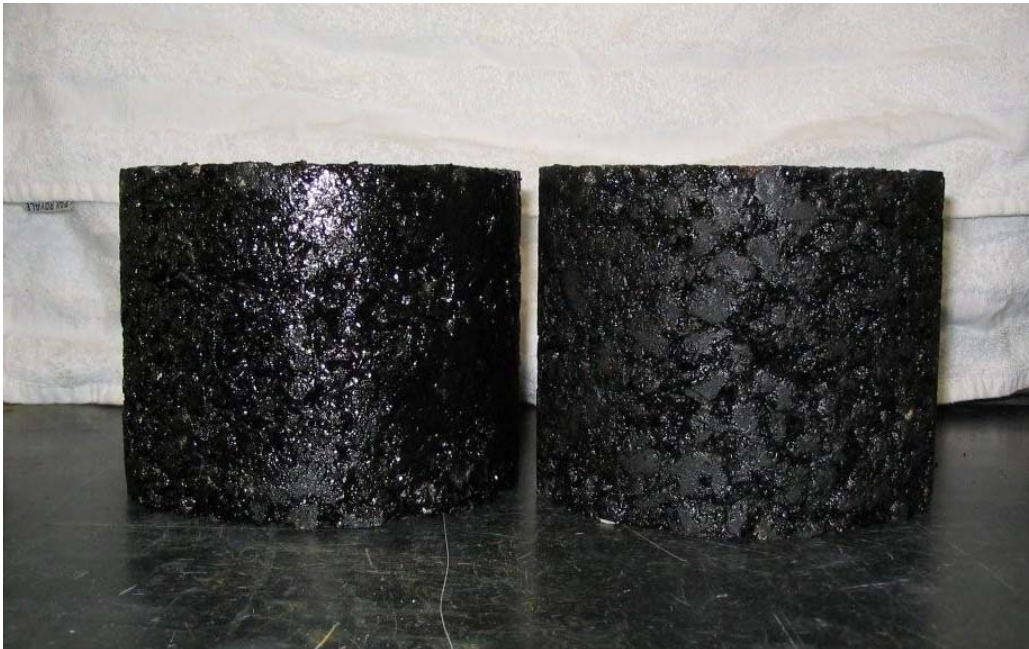
Figure 1. Sample with Fiber (Right) and without Fiber (Left) at Optimum AC%
