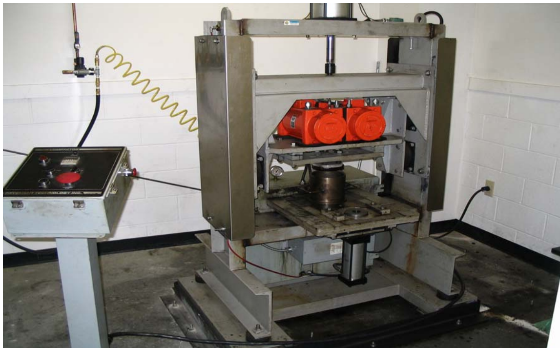
Figure 3. Vibratory Compactor used for Compaction of Test Samples.
