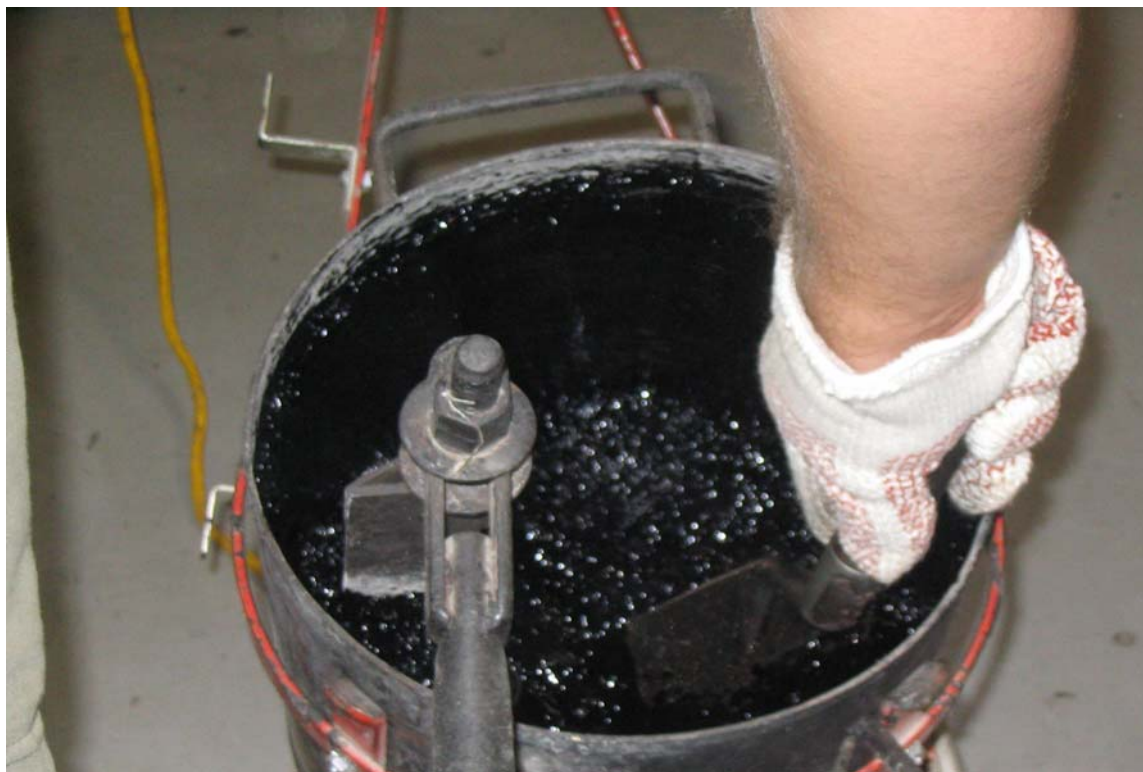
Figure 6. Hot Mix Asphalt in Bucket Mixer.
