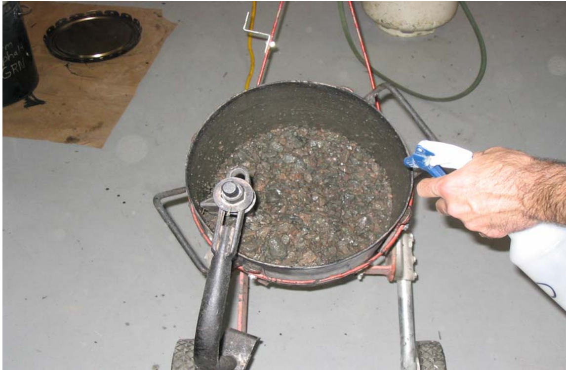
Figure 4. Introduction of Moisture to Aggregate for TSR Samples.
