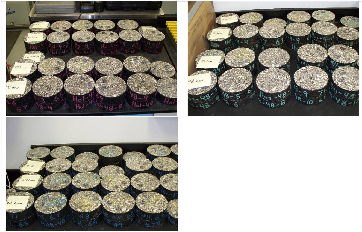
**Figure 3.41 Laboratory Samples Prepared for DC(t) Testing from the Three Binder Sources.**
