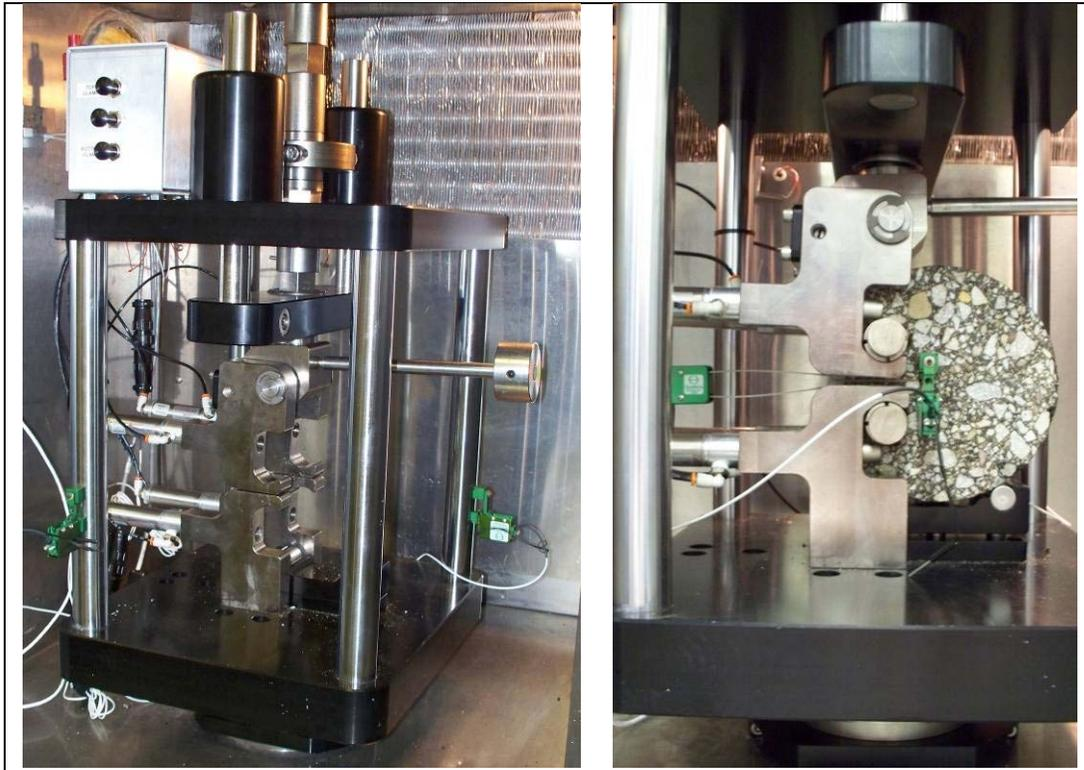
**Figure 3.42 Cox and Sons DC(t) Testing Device without sample (left) and with sample loaded (right) and instrumented.**
