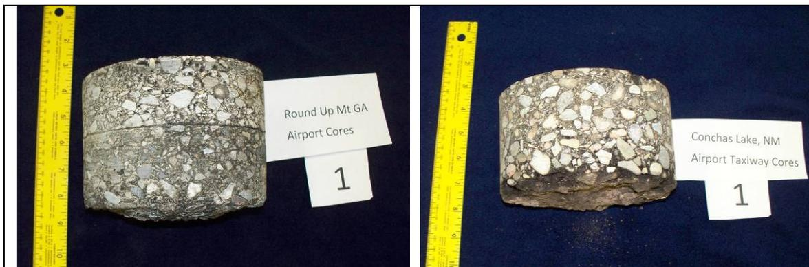
**Figure 4.2 Samples Cores from Roundup, MT (RPX) and Conchas Lake, NM (E89)**
