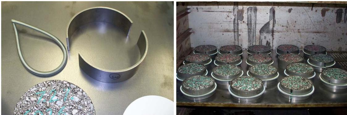
**Figure B.3 Long-term oven aging of laboratory compacted samples**
