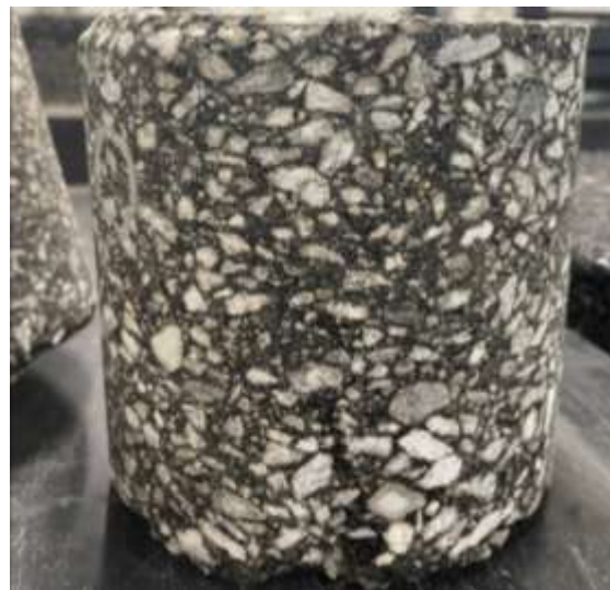
Figure 10. Closeup of Cores Extracted in Section S8 in Distress Area
