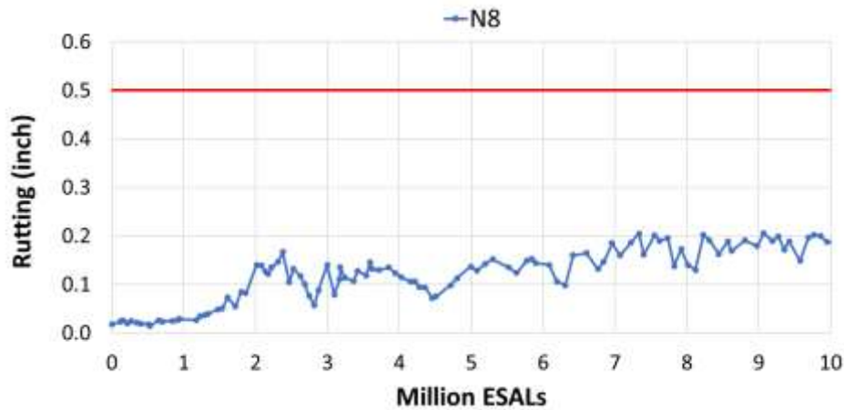
FIGURE 12 Field rutting data of Section N8.
