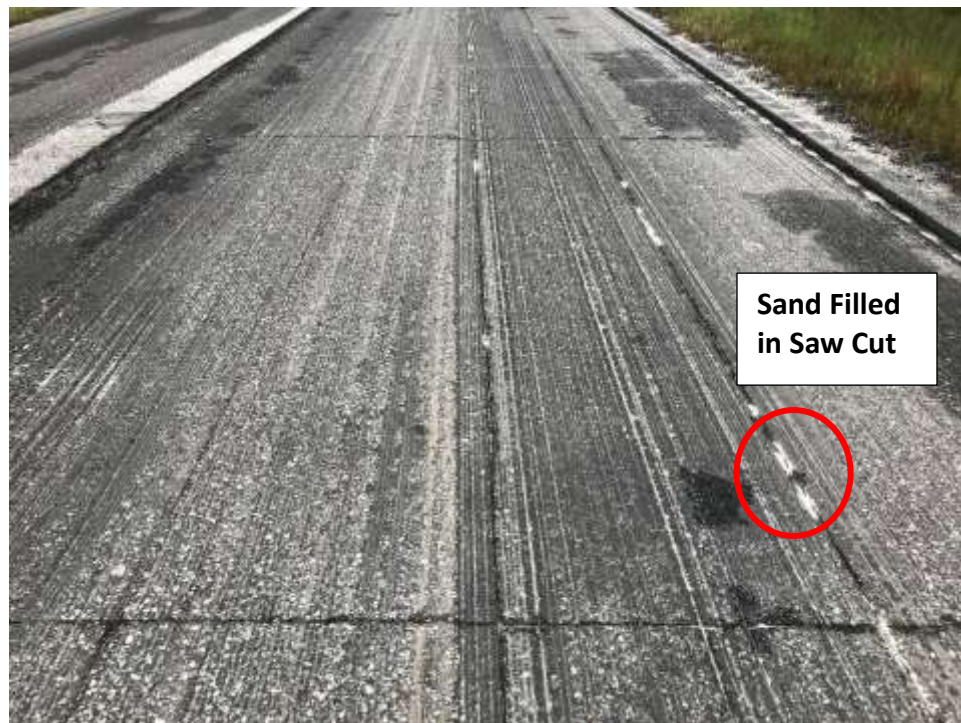
FIGURE 1 Deep saw cuts to simulate pavement cracks.
