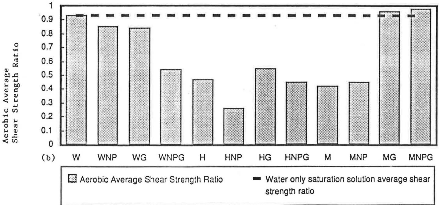
Figure 3: Histogram Illustrating the Relationship Between Average Shear Strength Ratio, Type of Preconditioning of Specimen, and Specimen Storage Environment.
