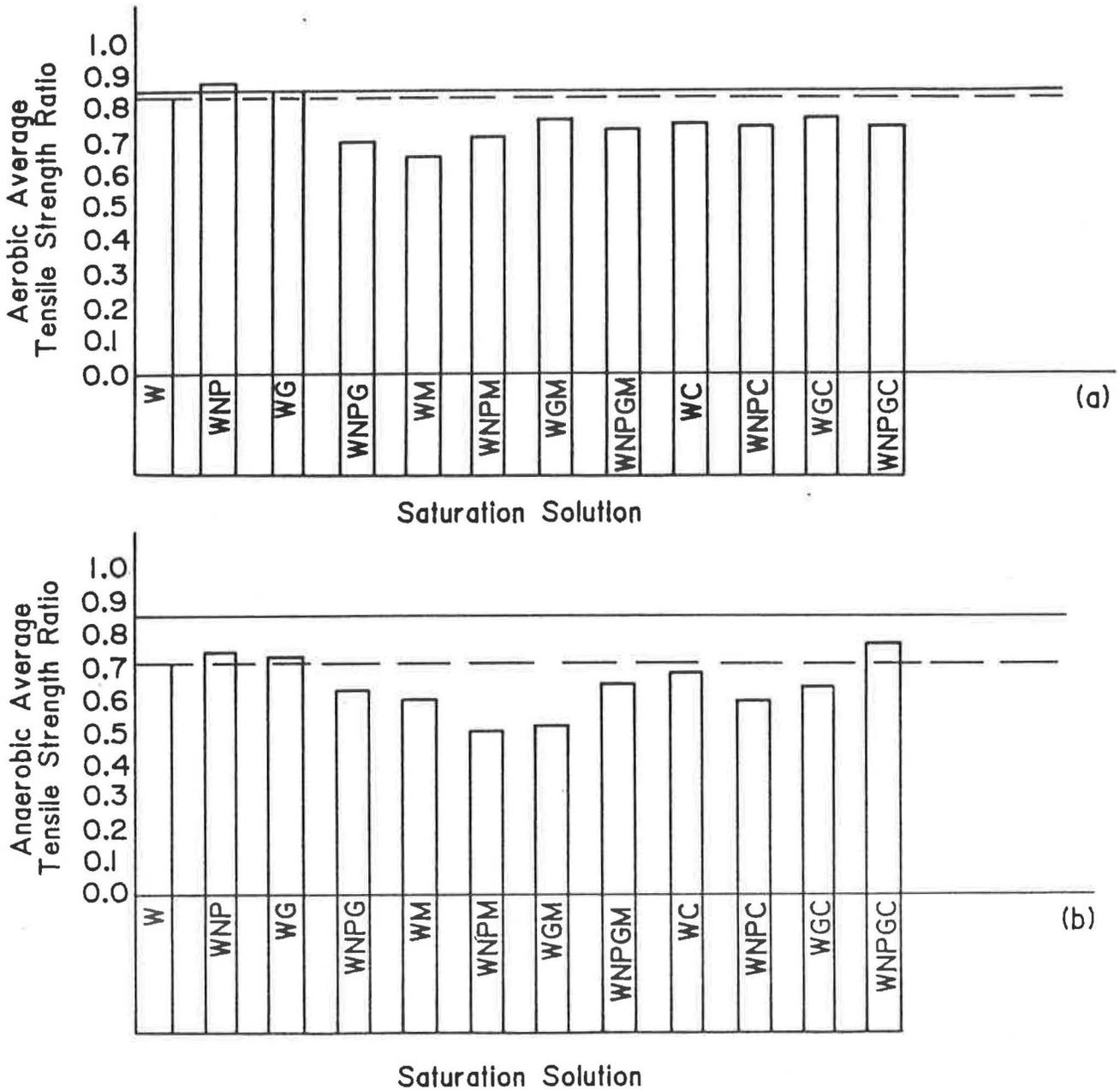
Figure 1: Histogram illustrating the Relationship Between Tensile Strength Ratio, Type of Saturation Solution, and of Storage Environment.
