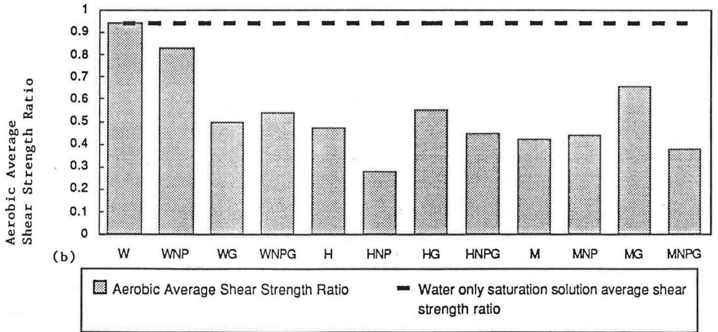
Figure 4: Modified Data Histogram Illustrating the Relationship Between Average Shear Strength Ratio, Type of Preconditioning of Specimen, and Specimen Storage Environment.
