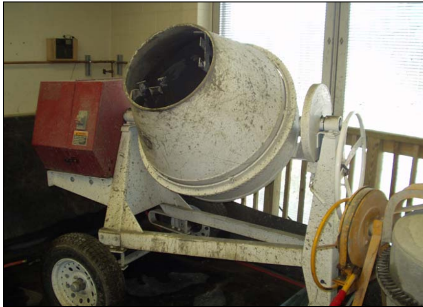
Figure 4.2: 12-ft 3 concrete mixer
