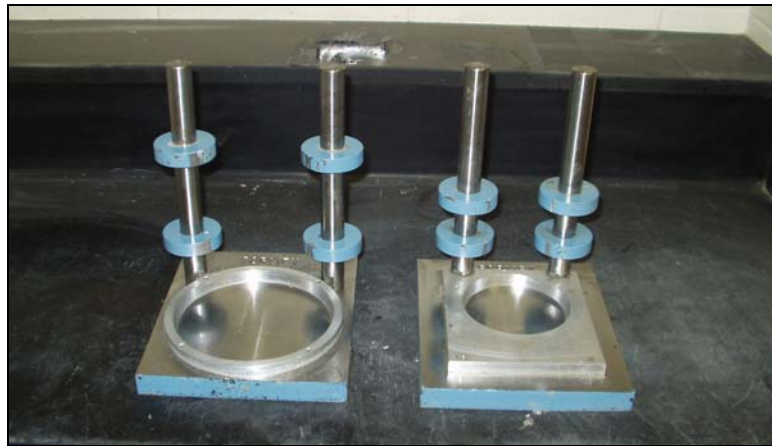
Figure 4.3: Molds used for sulfur capping
