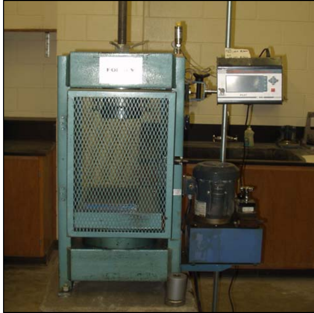
Figure 4.4: 400-kip Forney compression testing machine
