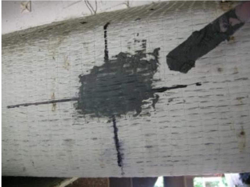
Figure M.5: Strain gage installation—application of solid epoxy
