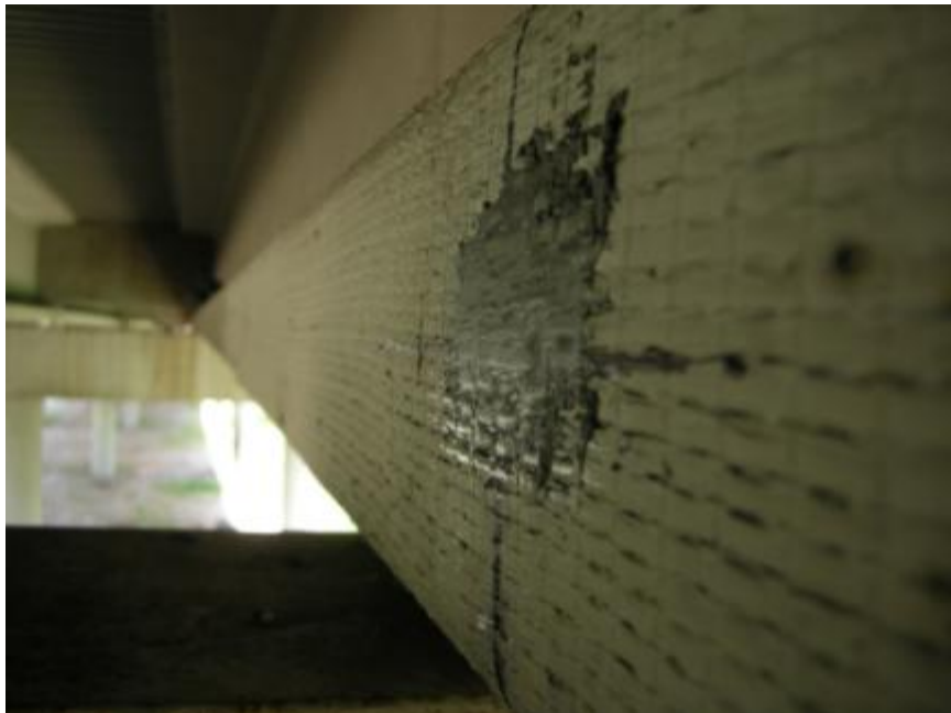
Figure M.6: Strain gage installation—epoxy surface
