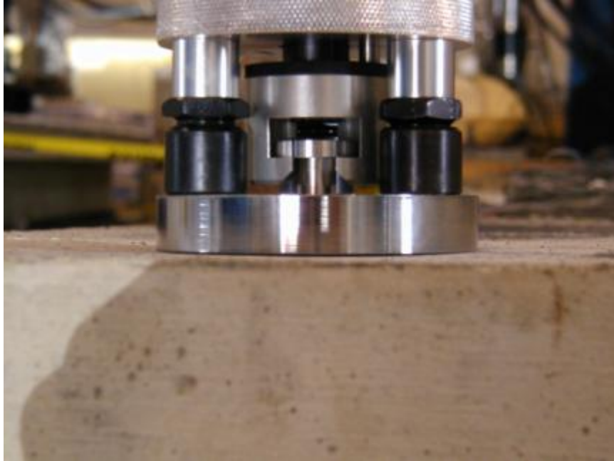
Figure 2.34: Adhesion test equipment (Swenson 2007)
