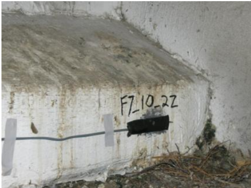
Figure 3.34: Strain gage installation—mastic tape for mechanical protection
