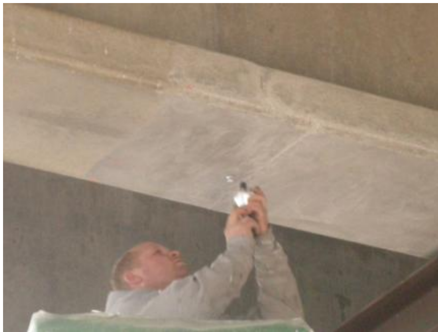
Figure 2.35: Performance of on-site adhesion test
