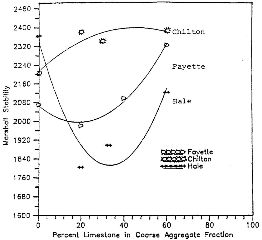
Figure 1. Marshall stability versus percent limestone in the coarse aggregate fraction.
