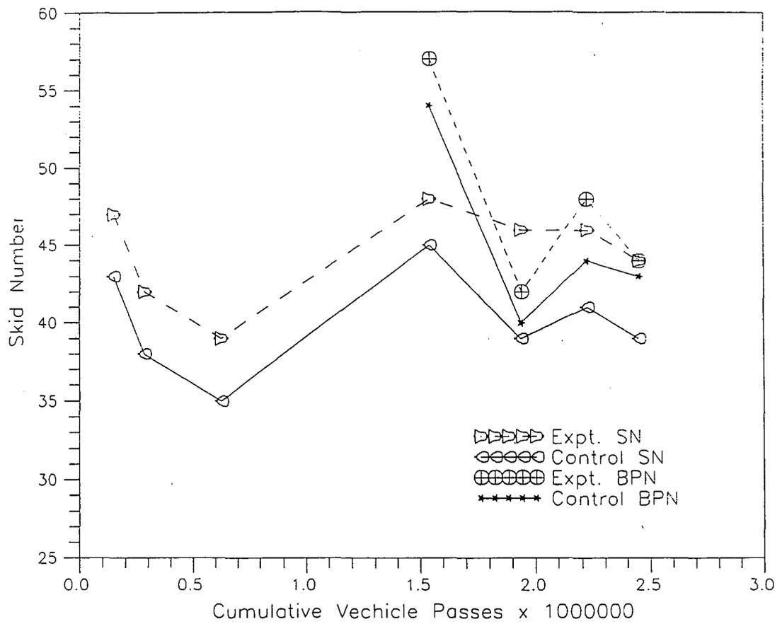
Figure 3. SN versus cumulative vehicle passes (Chilton County)
