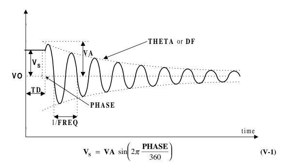
The shape of the waveform is described by the following equations:
