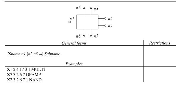
Subcircuits are specified in SPICE by using pseudo-elements beginning with the letter  $\mathbf{X}$ , followed by the circuit nodes  $n1 \ [n2 \ n3 \ ...]$  to be used in expanding the subcircuit and the name *Subname* of the subcircuit. The subcircuit is defined by the **.SUBCKT** statement. The number of nodes in the subcircuit call ( $\mathbf{X}$  statement) must be the same as in the subcircuit declaration (**.SUBCKT**).
