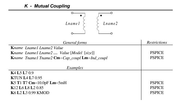
The mutual coupling statement describes a mutual inductive coupling between two inductors. *Lname1* and *Lname2* are the names of the two coupled inductors, and *Value* is the coupling coefficient K which must be greater than 0 and less than or equal to 1. Using the dot convention, place a dot on the first node of each inductor. The relation between the coupling coefficient K and the mutual inductance is given by:
