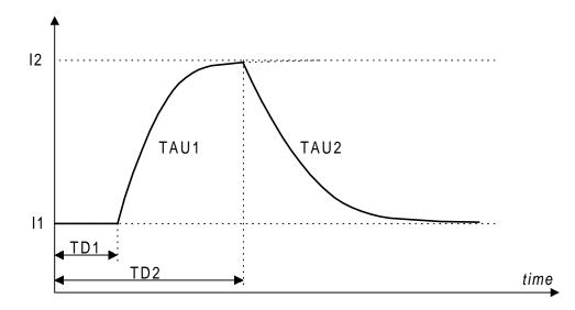
The shape of the waveform is described by the following equations:
