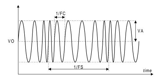
The SFFM (single-frequency frequency-modulated) waveform is described by the following equation:
