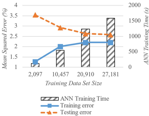
Fig. 7 Increasing ANN training data typically increases ANN accuracy, but large training data sets make ANN training difficult at the expense of increased training time
