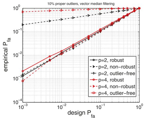
**FIGURE 2.** Empirical  $P_{fa}$  vs. design  $P_{fa}$  using the GLRT detector of Theorem 1, operating after data-cleaning (labeled “robust”), or on outlier-free data (labeled “outlier-free”), or on contaminated data (labeled “non-robust”): 10% proper outliers ( $p_o = 0.1$ ), vector median filtering used for cleaning,  $n = 256$ ,  $K = 15$ ,  $M = 8$ .
