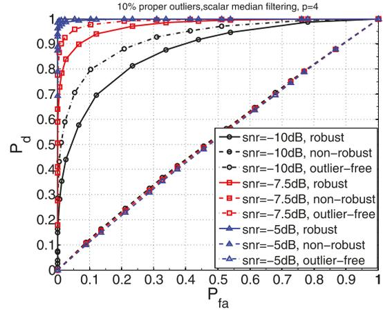
**FIGURE 5.** ROC curves using the GLRT detector of Theorem 1, operating after data-cleaning (labeled “robust”), or on outlier-free data (labeled “outlier-free”), or on contaminated data (labeled “non-robust”): 10% proper outliers ( $p_o = 0.1$ ), scalar median filtering used for data-cleaning,  $p = 4$ ,  $n = 256$ ,  $K = 15$ ,  $M = 8$ .
