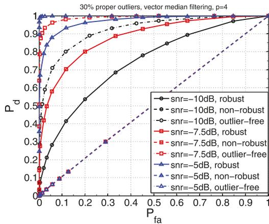
**FIGURE 7.** ROC curves using the GLRT detector of Theorem 1, operating after data-cleaning (labeled “robust”), or on outlier-free data (labeled “outlier-free”), or on contaminated data (labeled “non-robust”): 30% proper outliers ( $p_o = 0.3$ ), vector median filtering used for data-cleaning,  $p = 4$ ,  $n = 256$ ,  $K = 15$ ,  $M = 8$ .
