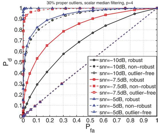
**FIGURE 6.** ROC curves using the GLRT detector of Theorem 1, operating after data-cleaning (labeled “robust”), or on outlier-free data (labeled “outlier-free”), or on contaminated data (labeled “non-robust”): 30% proper outliers ( $p_o = 0.3$ ), scalar median filtering used for data-cleaning,  $p = 4$ ,  $n = 256$ ,  $K = 15$ ,  $M = 8$ .
