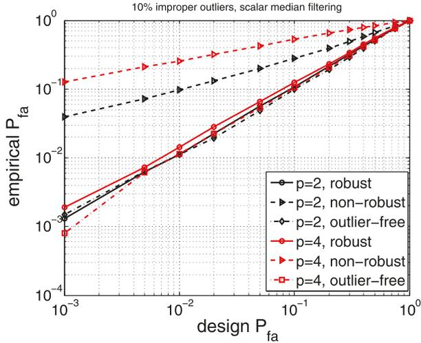
**FIGURE 3.** Empirical  $P_{fa}$  vs. design  $P_{fa}$  using the GLRT detector of Theorem 1, operating after data-cleaning (labeled “robust”), or on outlier-free data (labeled “outlier-free”), or on contaminated data (labeled “non-robust”): 10% proper outliers ( $p_o = 0.1$ ), scalar median filtering used for cleaning,  $n = 256$ ,  $K = 15$ ,  $M = 8$ .
