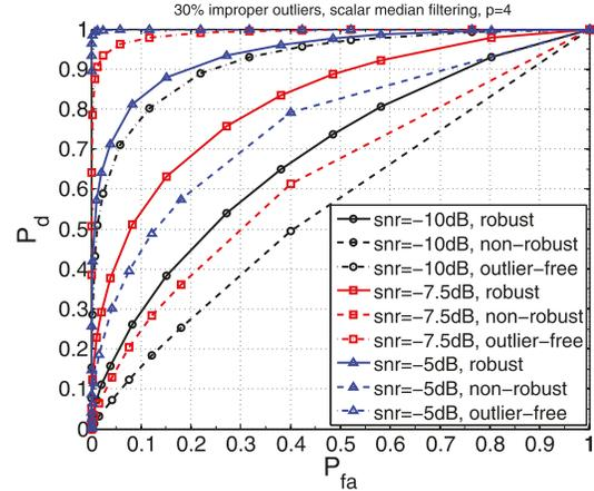
**FIGURE 8.** ROC curves using the GLRT detector of Theorem 1, operating after data-cleaning (labeled “robust”), or on outlier-free data (labeled “outlier-free”), or on contaminated data (labeled “non-robust”): 30% improper outliers ( $p_o = 0.3$ ), scalar median filtering used for data-cleaning,  $p = 4$ ,  $n = 256$ ,  $K = 15$ ,  $M = 8$ .
