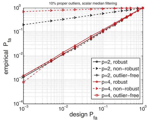
**FIGURE 1.** Empirical  $P_{fa}$  vs. design  $P_{fa}$  using the GLRT detector of Theorem 1, operating after data-cleaning (labeled “robust”), or on outlier-free data (labeled “outlier-free”), or on contaminated data (labeled “non-robust”): 10% proper outliers ( $p_o = 0.1$ ), scalar median filtering used for cleaning,  $n = 256$ ,  $K = 15$ ,  $M = 8$ .
