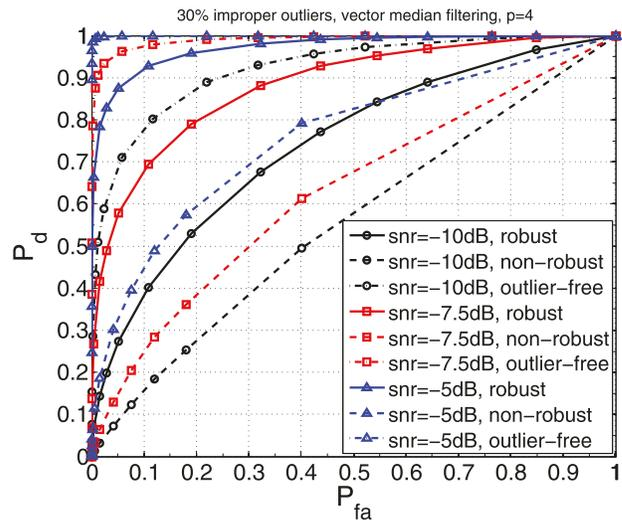
**FIGURE 9.** ROC curves using the GLRT detector of Theorem 1, operating after data-cleaning (labeled “robust”), or on outlier-free data (labeled “outlier-free”), or on contaminated data (labeled “non-robust”): 30% improper outliers ( $p_o = 0.3$ ), vector median filtering used for data-cleaning,  $p = 4$ ,  $n = 256$ ,  $K = 15$ ,  $M = 8$ .
