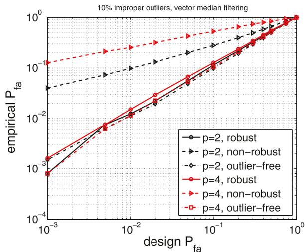
**FIGURE 4.** Empirical  $P_{fa}$  vs. design  $P_{fa}$  using the GLRT detector of Theorem 1, operating after data-cleaning (labeled “robust”), or on outlier-free data (labeled “outlier-free”), or on contaminated data (labeled “non-robust”): 10% proper outliers ( $p_o = 0.1$ ), vector median filtering used for cleaning,  $n = 256$ ,  $K = 15$ ,  $M = 8$ .
