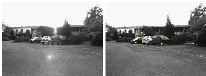
Fig. 17. Sun shines into the camera in the reference image (left) of experiment 4 but not in the current image (right) during navigation.
