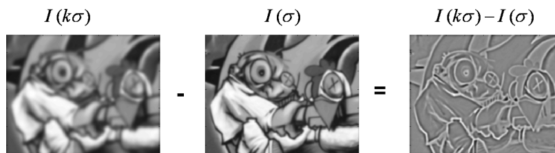
Fig. 6.1 The Laplacian can be approximated as a difference of two Gaussian smoothed images.
