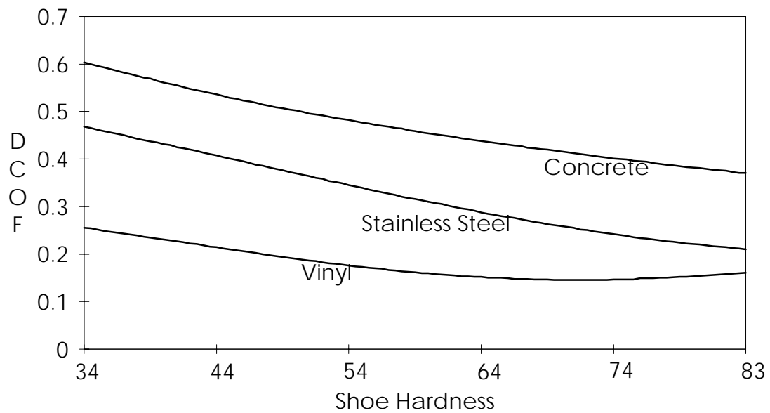
Figure 10. Response of DCOF as Shoe Hardness Changes for Concrete, Vinyl Tile and Stainless Steel Floors Contaminated by Oil When Force = 40N and Heel Contact Angle = 5°.
