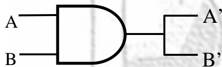
Wired-AND fault model
