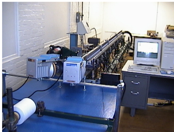
Figure 1 Air-jet filling insertion simulator developed at Auburn University
