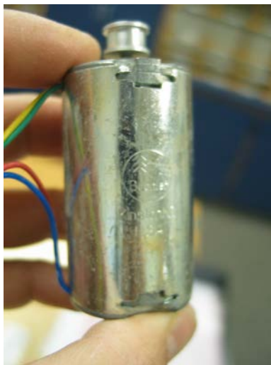
Figure 4. Buehler permanent magnet dc motor with tachometer
