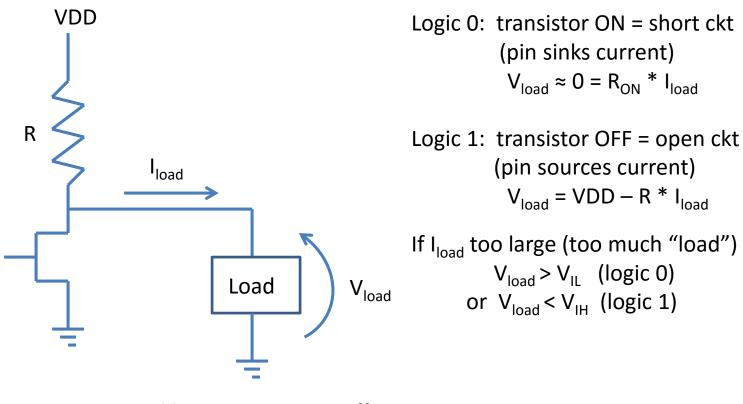
Load has: Resistance - affects I<sub>load</sub> Capacitance – affects V<sub>load</sub> rise/fall times
