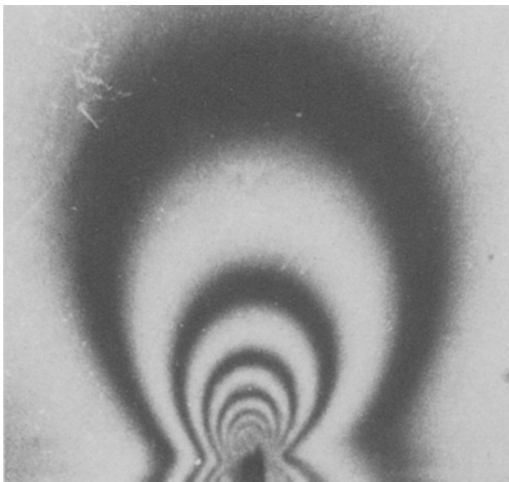
Fig. 10—Isochromatic patterns for the plate model with crack under pure Mode II deformation
