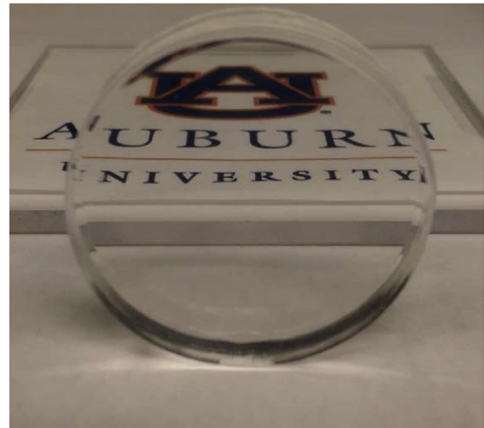
Fig. 8. Hollow metal tube (top) to punch out circular disk specimen and the resulting transparent disk shaped gel specimen (bottom).
