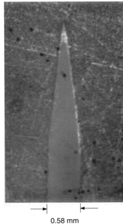
Fig. 5. Magnified view of the crack tip created using a sharpened blade
