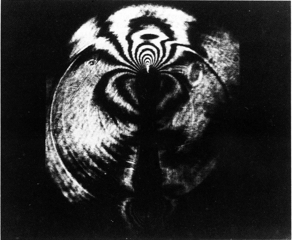
FIG. 23. Reflection mode x_1 -gradient CGS fringe pattern for a rapidly propagating crack in AISI 4340 steel specimen (MD-3) showing strong influence of stress waves.
