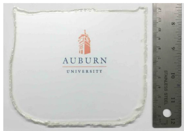
Fig. 4. A clear and sharp photograph of Auburn University logo through the cast specimen of a select (70:30 CoP:PU) grade-1 graft-IPN.
