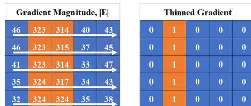
Fig. 20 Original gradient values (left) with arrows showing the general direction along which maximum values are determined, resulting in the thinned matrix (right)
