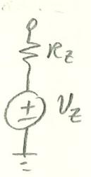
Zener Diodes → diodes made to take advantage of the Zener breakdown
