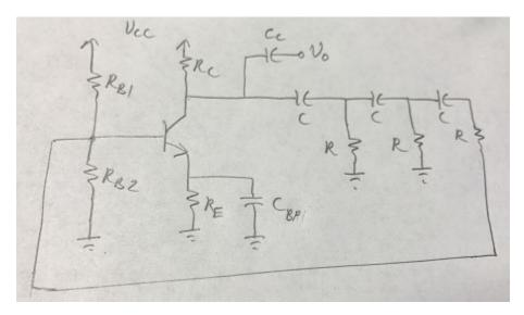
This circuit uses a common emitter (large negative gain) amplifier. The oscillator uses negative feedback to satisfy the BSC:  $1|-180^{\circ}$ .
