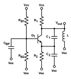
$C_{BP}$  is a bypass capacitor (assume an open for DC analysis and a short for small signal AC analysis)
