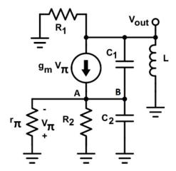
We will break the loop between nodes A and B to calculate the loop gain, AB. The BSC is satisfied when:
