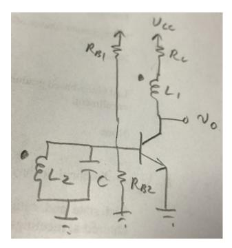
Same oscillator with possible biasing resistors shown.
