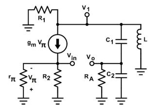
The three voltage nodes,  $V_{in}$ ,  $V_o$ , and  $V_1$ , are used to calculate the loop gain, AB. A is therefore defined as:
