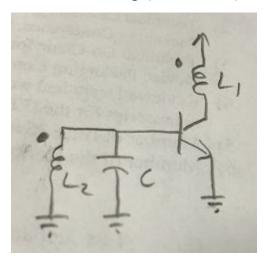
Without biasing resistors shown. The transformer provides feedback from the output of the common emitter amplifier back around to the base. A transformer can easily provide a 180° phase shift. Transformer's inductance with C determines the oscillation frequency.
