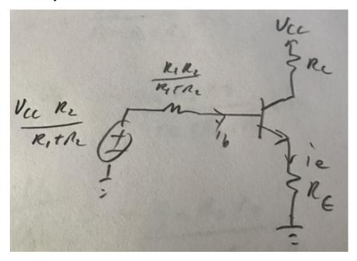
$$\frac{V_{cc}R_2}{R_1 + R_2} = I_E R_E + 0.7 + I_B \frac{R_1 R_2}{R_1 + R_2}$$
