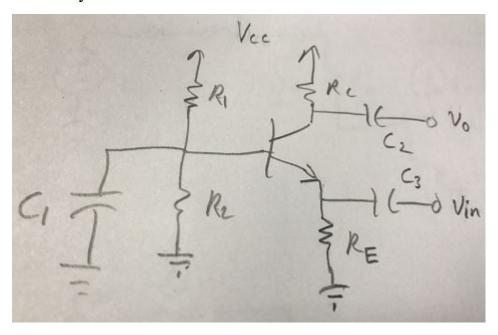
$C_1$ ,  $C_2$  and  $C_3$  are coupling capacitors
