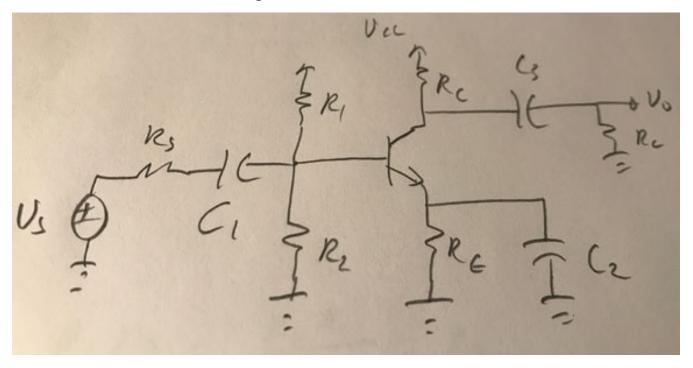
$C_1$ ,  $C_2$  and  $C_3$  are coupling capacitors: consider them to be open for DC analysis and shorts for higher frequency small signal analysis.
