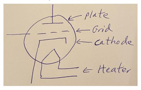
The background pressure inside the vacuum tube might be on the order of  $1x10^{-9}$  atm.
