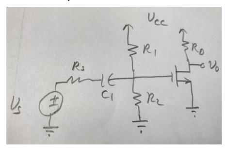
$C_1$  is a coupling capacitor: an open for the DC analysis.
