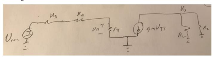
$$R_b = \frac{R_1 R_2}{R_1 + R_2}$$
