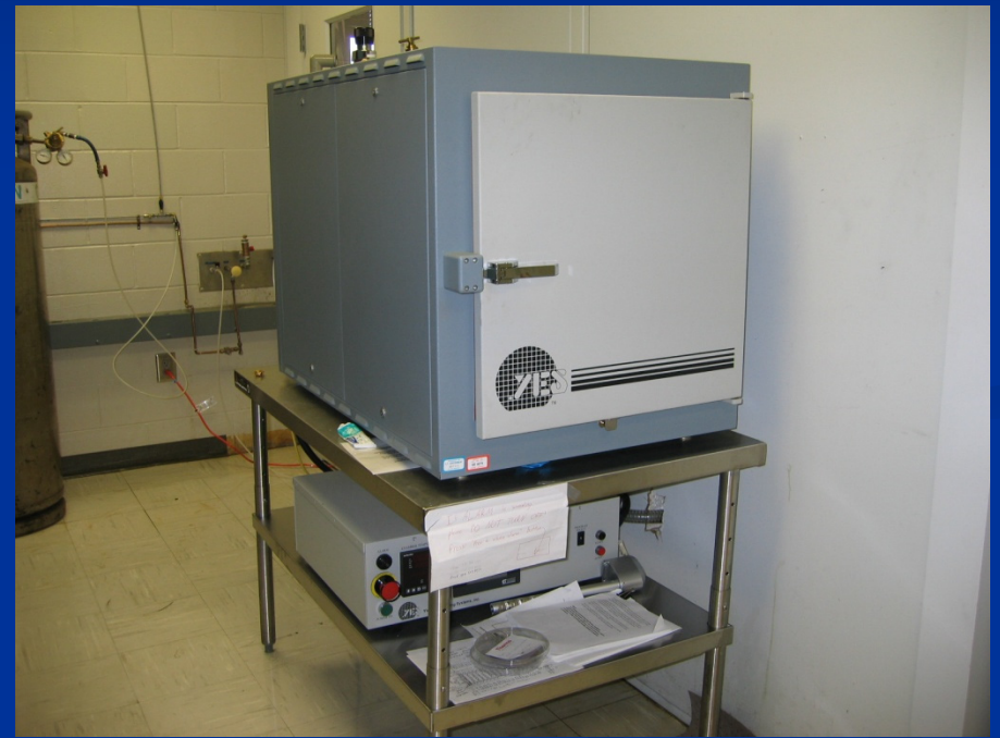
Polyimide Vacuum Curing Oven
