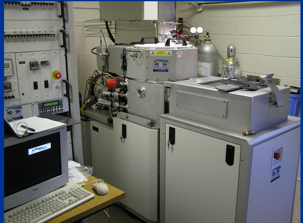
STS ASE Bosch Process Si DRIE Etcher
