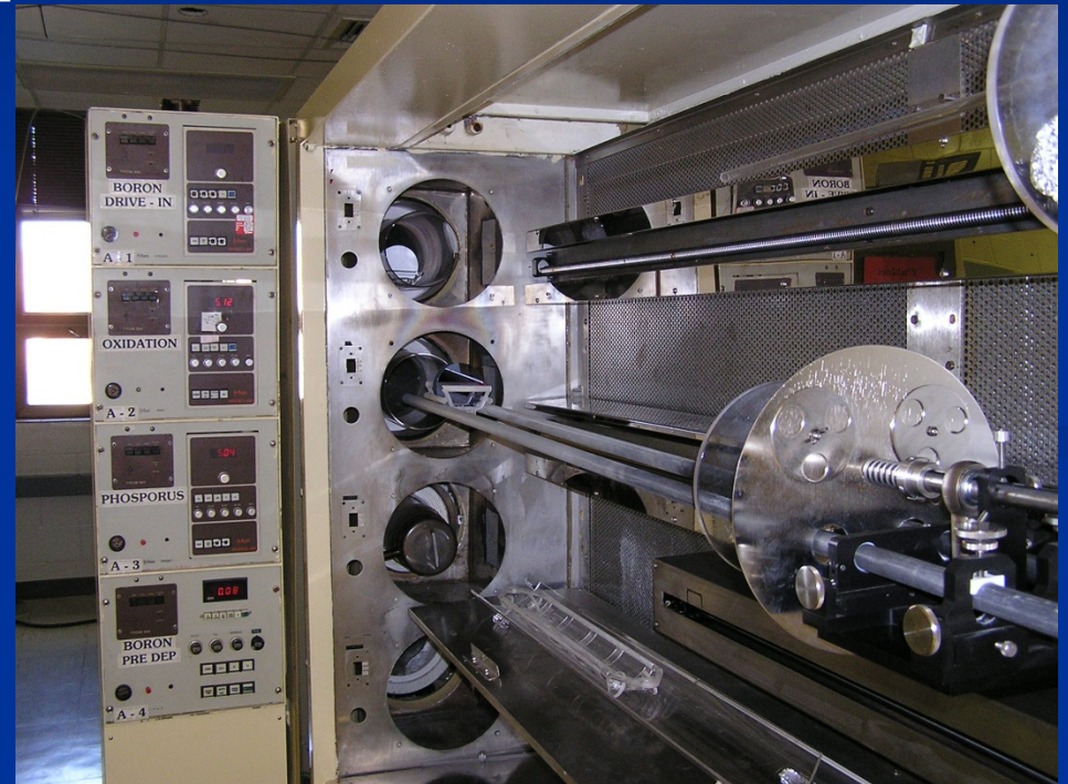
Oxidation and Diffusion Furnace
